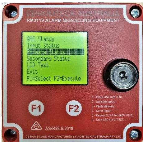
Image: Selecting Primary Signal Test
