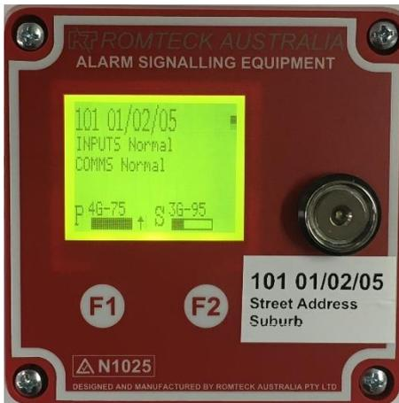
Image: An ASE 3118 in Normal mode with no active alarms
