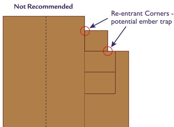
Diagram showing comparison of building and roof shapes
