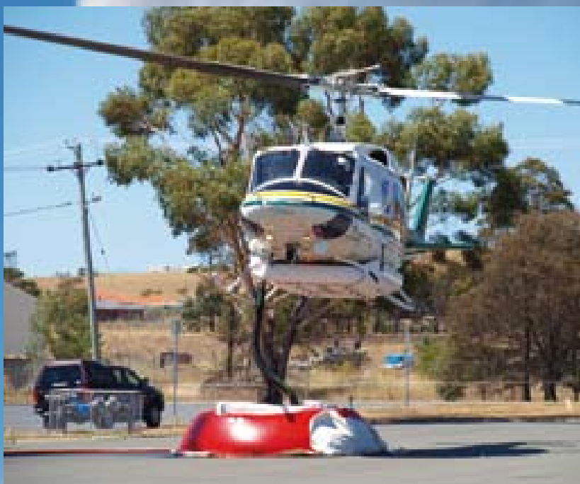
721 filling – 1400 litres in 35 seconds
