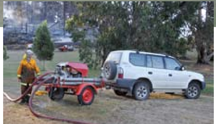
The trusty Penguin VW trailer pump boosting supply from the hydrant 1 km away
