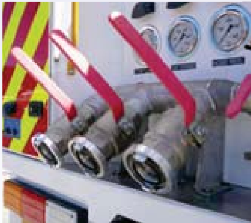
Rear view of a 2008 model pumper tanker incorporating Storz couplings
