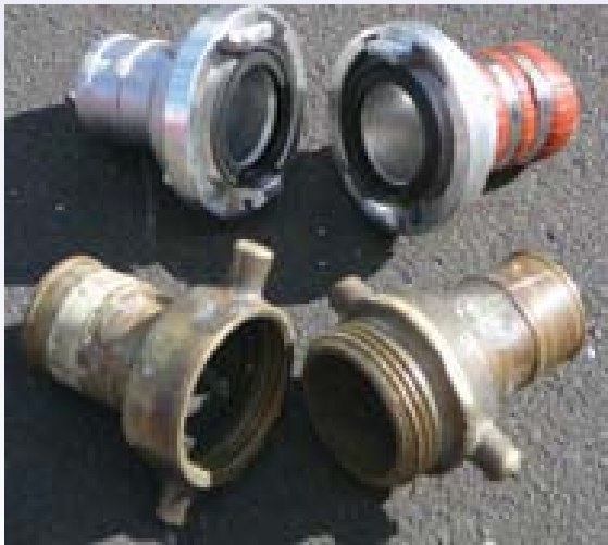
Male and female 64mm traditional hose tail set as well as the new Storz 2 1/2 inch coupling set
