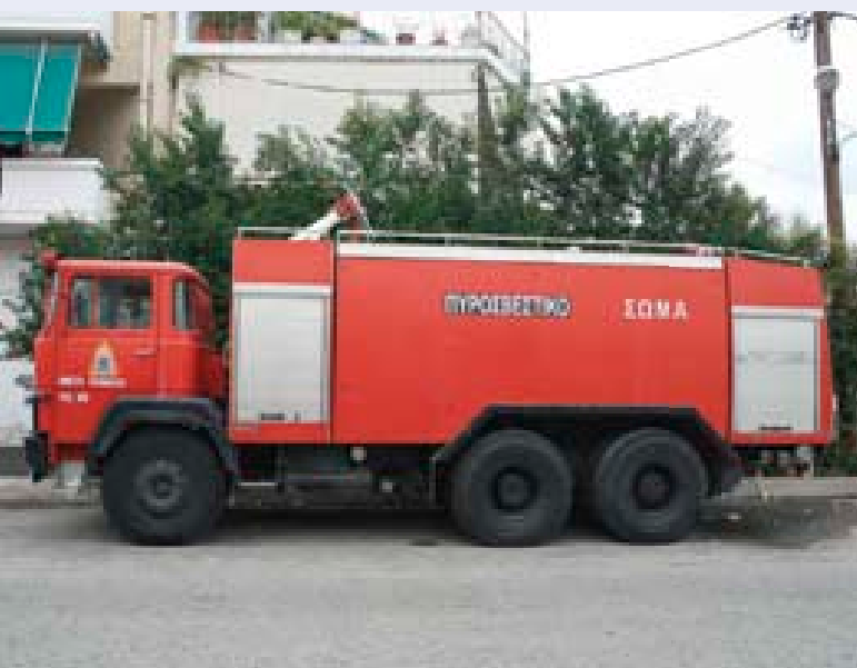
Hellenic Fire Brigade 10,000 litre tanker pre positioned to provide static water supplies
