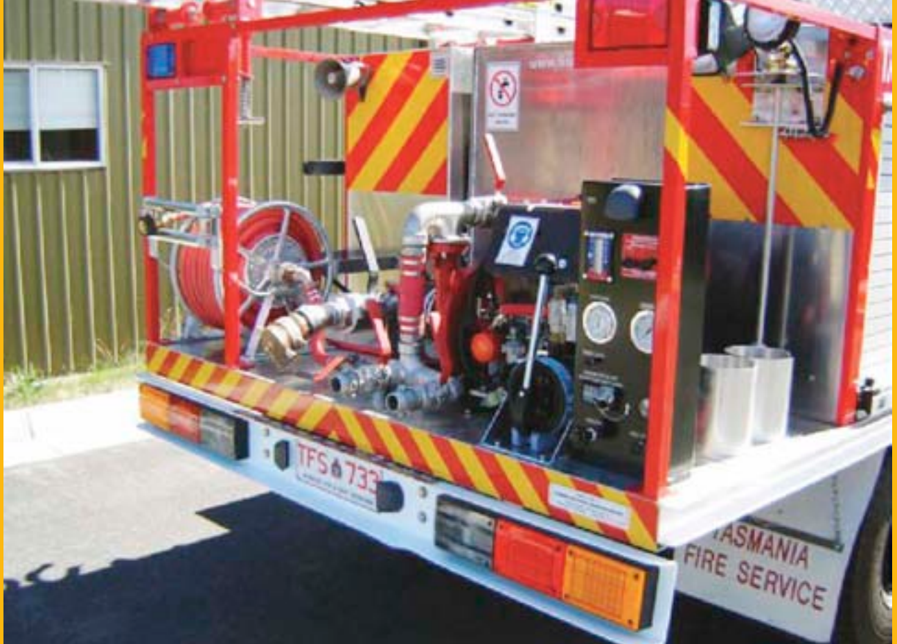
Extended chassis, increased deck storage area allowing increased water capacity and reduced front axle loadings
