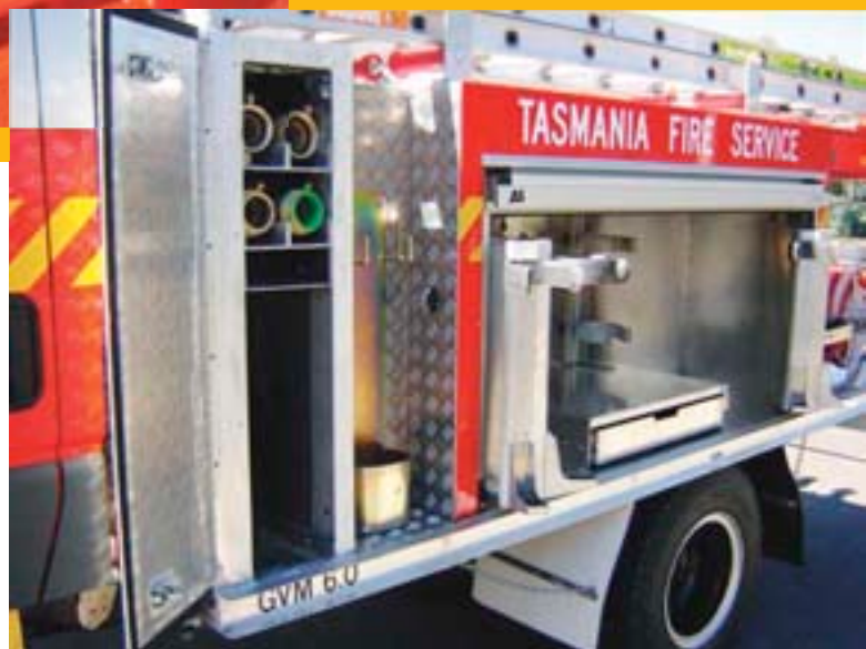
Increased locker capacity allowing all equipment to be accessed from ground level
