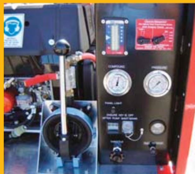
LED tank level indicator, ignition, throttle and stop
