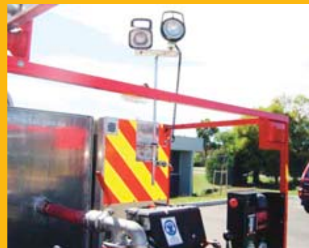
360° stem light incorporating gas discharge scene light.
