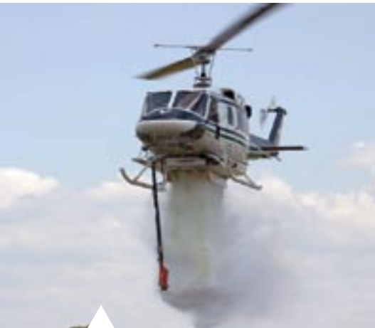
Helitack 721 (Bell 212) in Bellytank mode delivering 1400 litres of water/foam
