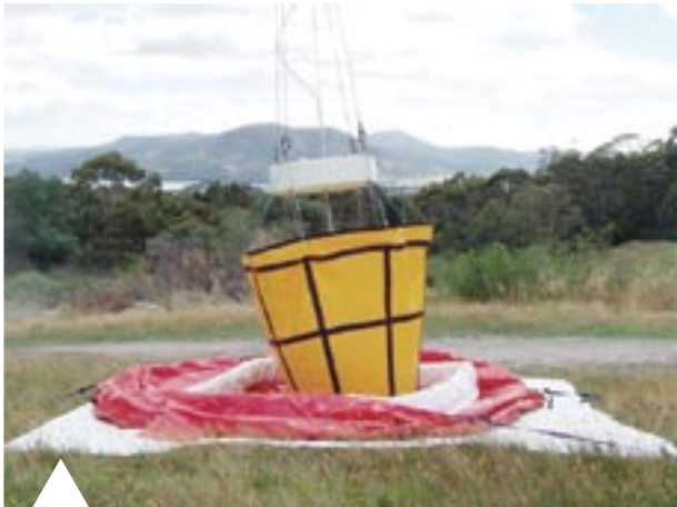
7500 litre Buoywall Dam being filled by a helicopter to provide a water source for refilling tankers
